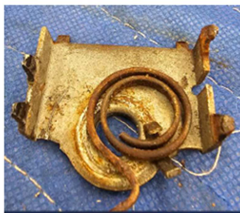
Dismantle the thing a find the broken spring.
